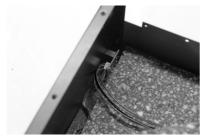
7. Place the plate K on the back cover centered to the sides, leaving a gap of 7 mm on both sides and taking care that it rests on the connectors. Strong press the plate to fix well.
